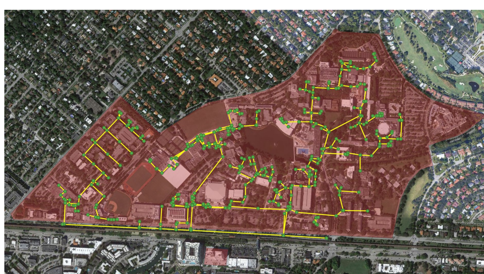
Figure 2. The layout of the Gables campus sewer lines that were sampled.
